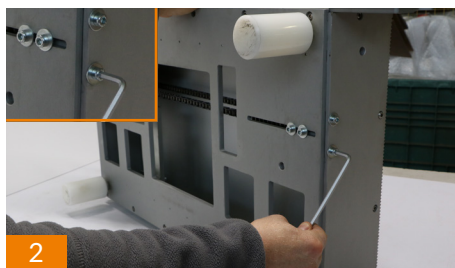
2 Tension the chain by tightening the screws with the provided spanner and paying attention to equally rotate both the screws.
